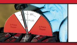
A TWO-PIECE STEM AND REPAIR UNIT, AND THEN 2 A TWO-PIECE STEIN AND THE ATT STATUS BONDED TOGETHER DURING THE REPAIR PROCESS. This works well when the angle of the injury exceeds 25 degrees.
