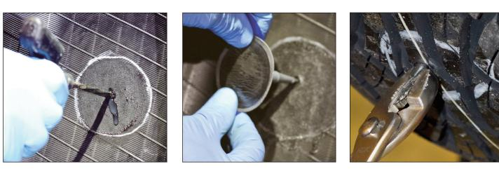
**NOT ALL TIRES CAN BE REPAIRED.** Check with the manufacturer for specific guidelines such as run flat technology tires, and commercial service applications.
